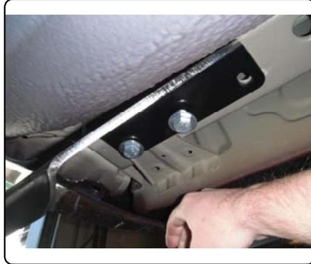
4. On the driver side frame rail fishwire a 7/16-14 x 1 1/2" carriage bolt and CM-SP2 spacer through the access hole and into the existing hole in the bottom of the frame rail. Secure with 7/16" flange nut.
