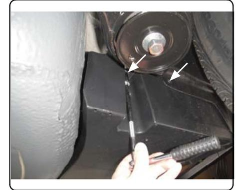
2. Locate (2) weldnuts near the end of each frame rail. Clean weldnuts of debris and rust to ease hitch installation.
