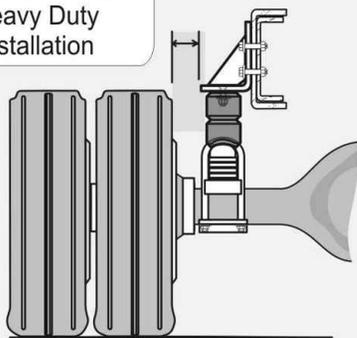
Check clearance when Vehicle is Empty
