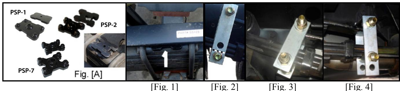
**Step 4:** While there is no designated front or rear side / left or right side, its best to insert spring with the eye bolts threads facing outward. Position the SuperSprings directly on top of the Poly Spring Pad. [Fig. 1]
