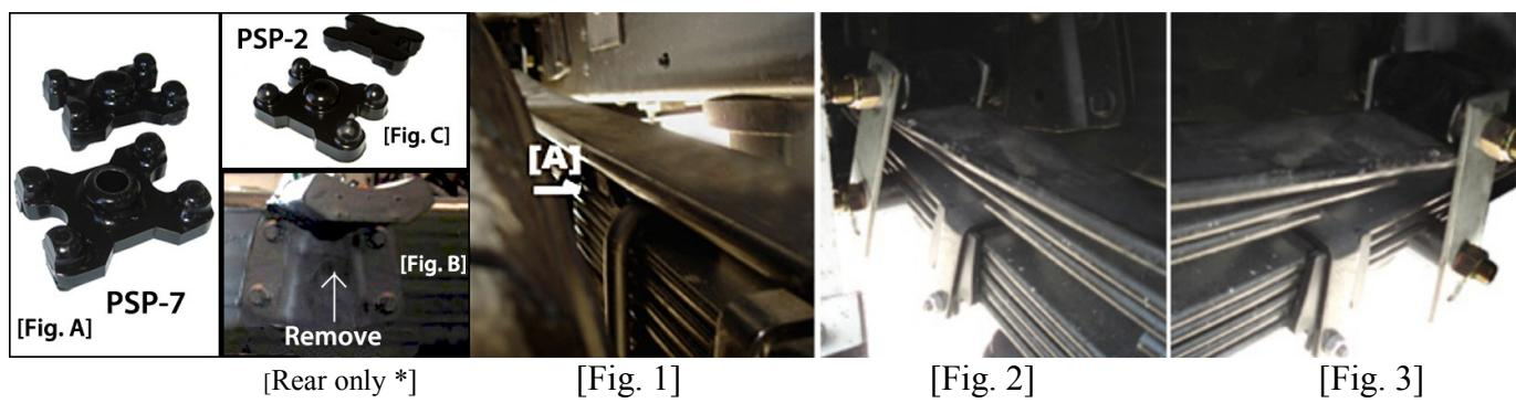
**Step 4:** While there is no designated front or rear side / left or right side, its best to insert spring with the eye bolts threads facing outward. Initially roughly center it directly on top of the PSP. [Fig. 1]
