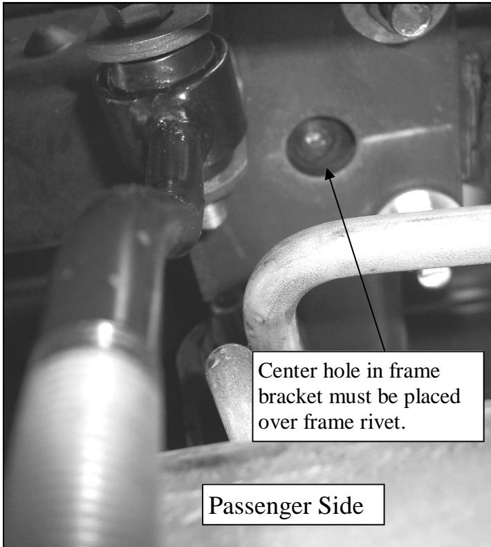
10. Adjust end links so that the arms of the sway bar are parallel with the ground. When satisfied with fit, attach end links to the rearmost hole of sway bar with 7/16 x 2-3/4 bolts, washers, and locknuts. On the passenger side install a spacer between the sway bar and end link bushing to provide tailpipe clearance.
