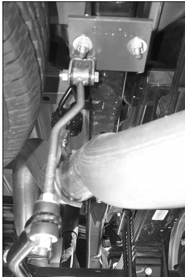
7. Thread locknut on to threads of end link far enough to mount flat washers and bushings to the end of sway bar as shown in photo three (3). Attach sway bar to end link using locknuts provided in kit. **LEAVE LOOSE AT THIS TIME** to allow for adjustment later.
