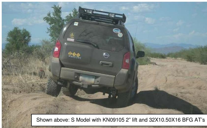
Shown above: S Model with KN09105 2" lift and 32X10.50X16 BFG AT's
