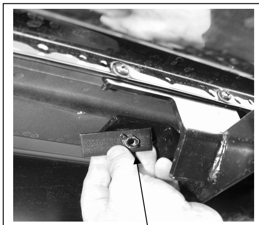
Fig 1. Note that nut should be installed facing up. Photo shows nut facing down
