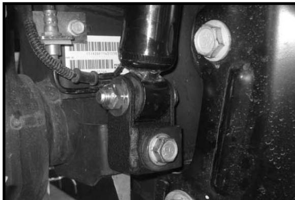
12. Working on the driver side, install the sway bar back to the sway bar end link and secure using the OE hardware. Make sure to use loctite and torque to **40 ft lbs.** Repeat procedure on the passenger side.
