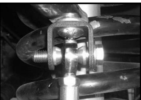
10. Locate (1) S10196 lower double sided threaded bracket, (1) 1/2" USS flat washers and (1) 9/16" unitorque nut from hardware bag 30927NB2. Install the new lower double side threaded bracket into the stock lower mount and secure using the new hardware. Make sure to use loctite and torque to **85 ft lbs**. **Special note: Use a 7/8"open ended wrench to hold the new lower bracket when torquing the 9/16" unitorque nut.**
