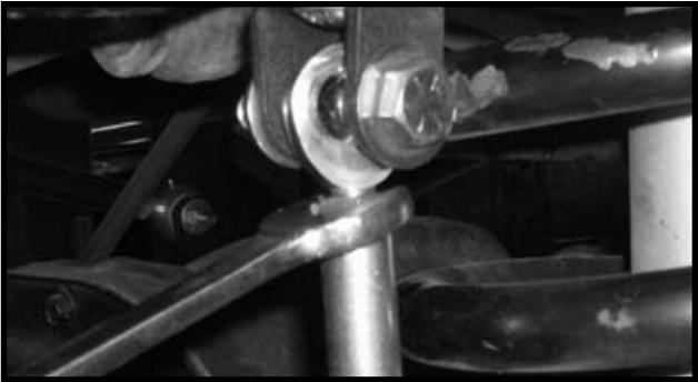
11. Locate (1) S10194 conned sleeves and (1) 1/2" unitorque nut from hardware bag 30927NB1. Install the new end link onto the previously installed lower double sided thread bracket. Now install the conned washer and secure the end link to the bottom bracket using the new 1/2" unitorque nut. Make sure to use loctite and torque to **55 ft lbs**. **Special note: Use a 7/8"open ended wrench to hold the new lower bracket when torquing the 7/16" unitorque nut.**
