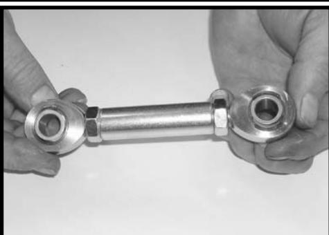
8. Locate (1) 1/2" x 2 1/2" bolt, (2) 7/16" flat washers, (1) 1/2" unitorque nut and (2) S10194 conned sleeves from hardware bag 30927NB1. Install the new all thread sleeve and hiem joints to the upper bracket using the new hardware and conned washer. Make sure to follow the photo's to properly install the conned sleeves. Make sure to use loctite and torque to **70 ft lbs**.
