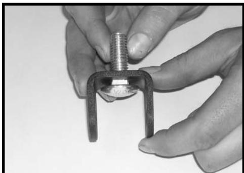
4. Locate (1) 9/16" flat washers from hardware bag 30927NB1 and install it on the new carriage bolt.
