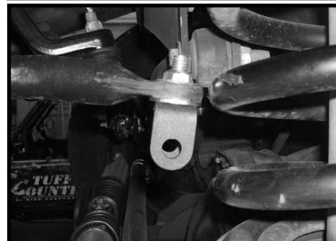
7. Locate (1) S10195 all thread sleeve and (2) S10116 hiem joints from hardware bag 30927NB1. Install the new hiem joints into each end of the new all thread sleeve.
