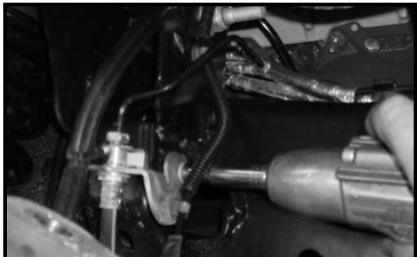
11. Working on the driver side, install the strut assembly back into the stock location, it may be necessary to pry down on the lower control arm in order for the lower eyelet of the shock to go into its pocket. Secure the strut using the stock bolt and hardware on the lower part, and using the new 3/8" nylon lock nuts and 5/16" flat washers on the upper mount. Torque the upper 3/8" hardware to **32 ft lbs** and the lower stock bolt to **100 ft lbs**. Repeat on passenger side.
