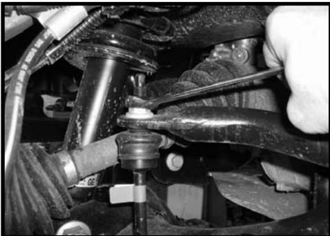
7. Working on the driver side, remove the nut and bolt holding the strut assembly to the lower control arm. Repeat on passenger side.
