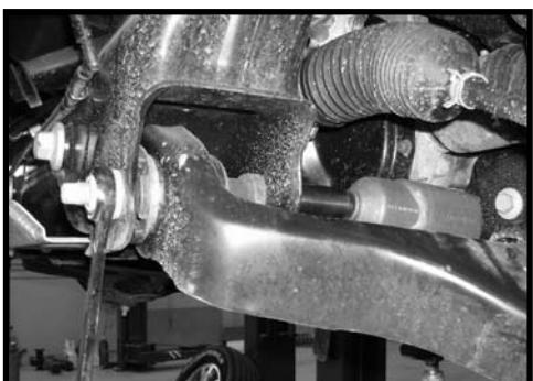
9. With both strut assemblies out of the vehicle it is time to install the new leveling spacers. Install these directly on top of the stock strut plate and secure them using the stock nuts. Torque to **35 ft lbs**.
