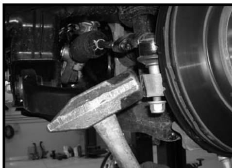
6. Working on the driver side, disconnect the sway bar end link from where it is connected to the sway bar, do not disconnect the end link from the lower control arm. Repeat on passenger side.
