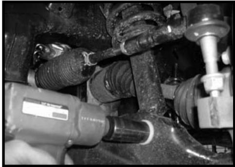
8. Working on the driver side, loosen but do not remove the (2) bolts holding the lower control arm to the vehicle. Repeat on passenger side. **Special note: This is done so that the lower control arm can swing down and allow you to remove the strut assembly from the vehicle. Also, the use of a pry bar may make removal easier.**
