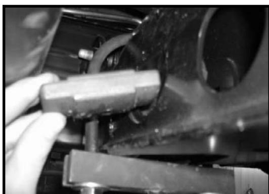
5. Working on the driver side, tap the stock torsion bar forward until the stock torsion bar key can be removed. Remove and discard the stock torsion bar key.
