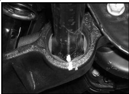
4. Working on the driver side and using a proper torsion bar removal tool. **Special note: Tuff Country EZ-Ride Suspension requires that a proper torsion bar unloading tool be used when performing this installation. If you do not have one, please contact your local GM dealer to purchase one from them.** Carefully remove the stock torsion bar bolt and block. Set the stock torsion bar bolt and block aside. Remove the stock torsion bar unloading tool from the stock cross member.
