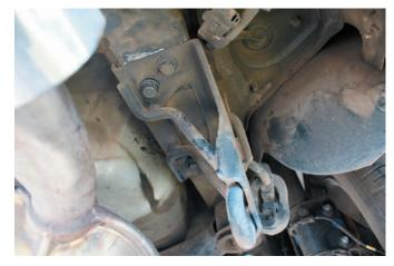
3. Remove the tow hook, four bolts on the passenger side.
