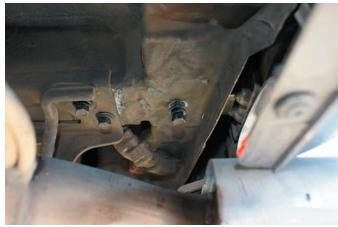
**4. On the** driver side, remove the two rear most bolts. There is a third weld nut on the driver side, you will be using it to install the hitch.
